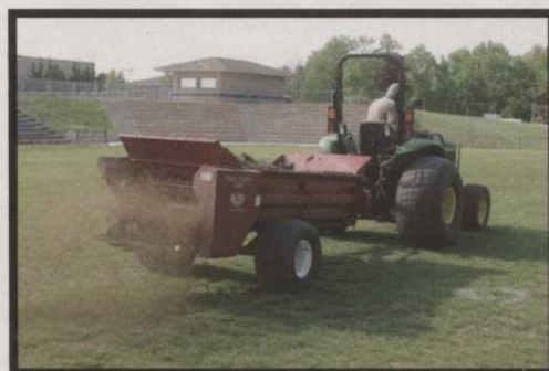
>> CORE CULTIVATION (above) coupled with sand topdressing ( below ) is a common practices for alleviating surface compaction and improve drainage. Photos provided by Alec Kowalewski and James Crum.
