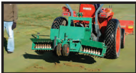
» IMAGE 3: Cultivation equipment that remove excessive organic matter accumulation include implements such as the Toro ProCore (top) and Graden (bottom). Photos courtesy of Alec Kowalewski.
