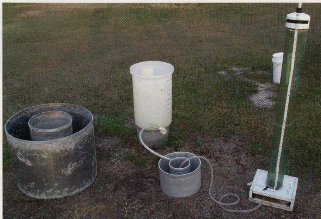
Photograph of 12-inch diameter (inner) and 24 inch diameter (outer) double ring infiltrometer (left/A); 6-inch diameter (inner) and 12 inch diameter (outer) double ring infiltrometer (center/B), and Mariotte siphon developed to maintain a constant inner head in the infiltration rings (right/C).
