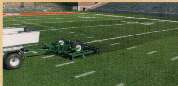
GreensSlicer Spring Tine Rake 3 rows of 28 tines.
