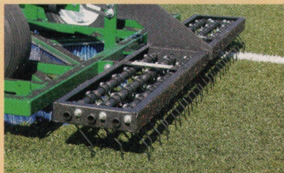
GreensSlicer Spring Tine Rake 3 rows of 28 tines.
