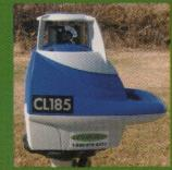
Excellent for use with a rod mounted receiver or machine control applications. With an adjustable range of flat to -1.85%, this laser is a sports field contractors most valuable tool.
