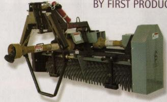
The VC-60 Verti-Cutter is designed for continuous heavy-duty operation on all sports fields in all types of turf. The unit has a "patented" swing hitch that allows the operator to turn while verti-cutting without tearing the established turf. Cutting depth on the VC-60 is easily adjusted in the field, without tools "up to 1 1/2 inches deep" using quick release pins on 3/16-inch increments.
