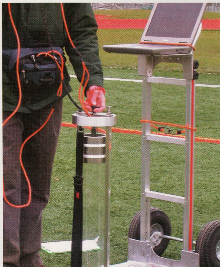
Figure 1A and 1B. Impact tester used for synthetic turf testing (A) and for natural turf and soil testing (B).
