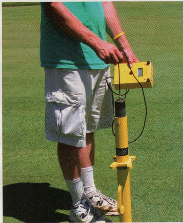
Figure 1A and 1B. Impact tester used for synthetic turf testing (A) and for natural turf and soil testing (B).
