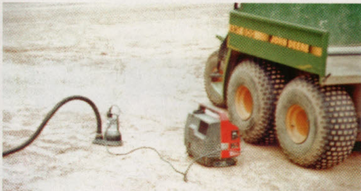
Power-generated sump pump with 3-inch deep and hose
