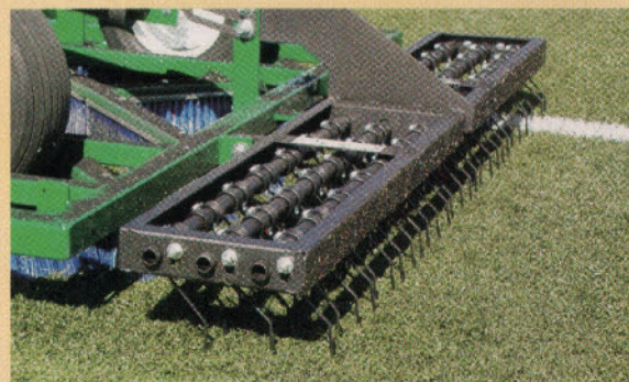
GreensSlicer Spring Tine Rake 3 rows of 28 tines.
