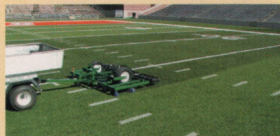
GreensSlicer Spring Tine Rake 3 rows of 28 tines.
