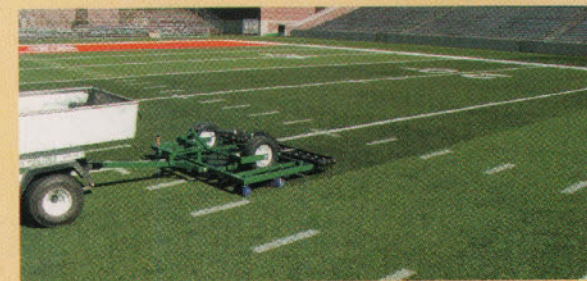
GreensSlicer Spring Tine Rake 3 rows of 28 tines.
