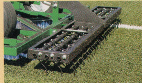
GreensSlicer Spring Tine Rake 3 rows of 28 tines.
