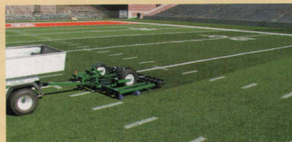
GreensSlicer Spring Tine Rake 3 rows of 28 tines.
