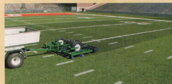
GreensSlicer Spring Tine Rake 3 rows of 28 tines.
