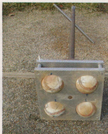
Devices used for measuring traction, static ball-to-surface friction, and dynamic ball-to-surface friction of skinned infield plots at the University of Connecticut.
