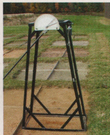
Devices used for measuring traction, static ball-to-surface friction, and dynamic ball-to-surface friction of skinned infield plots at the University of Connecticut.
