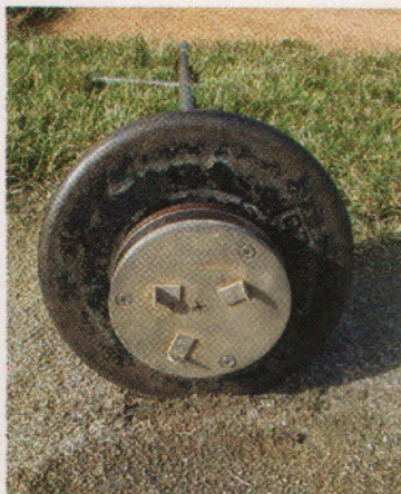
Devices used for measuring traction, static ball-to-surface friction, and dynamic ball-to-surface friction of skinned infield plots at the University of Connecticut.
