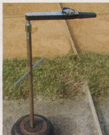
Devices used for measuring traction, static ball-to-surface friction, and dynamic ball-to-surface friction of skinned infield plots at the University of Connecticut.
