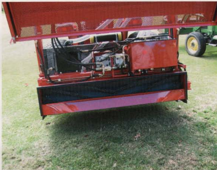
The Verti-Air machine blows high-speed air deep into the synthetic turf carpet, then a rotary brush picks up the dislodged infill material and debris and throws it on a filter, which returns the cleaned infill to the field.
