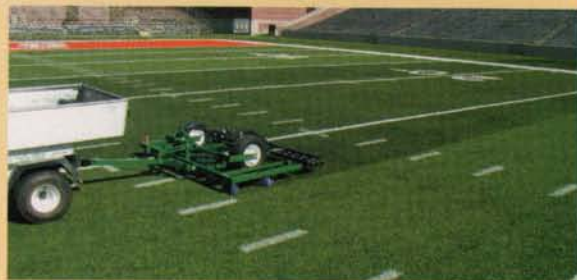
GreensSlicer Spring Tine Rake 3 rows of 28 tines.
