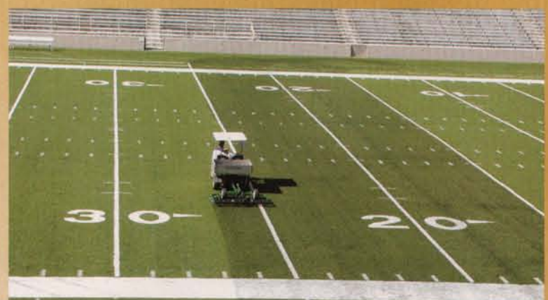
GreensSlicer Spring Tine Rake 3 rows of 28 tines.
