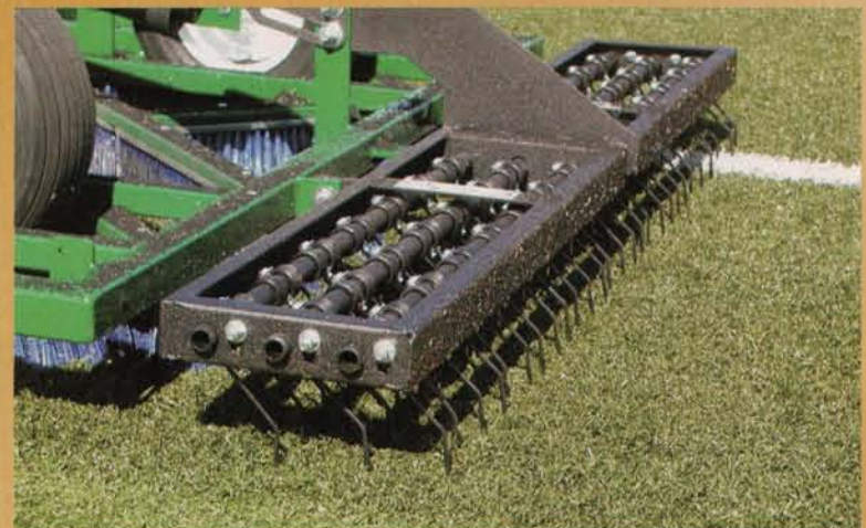
GreensSlicer Spring Tine Rake 3 rows of 28 tines.
