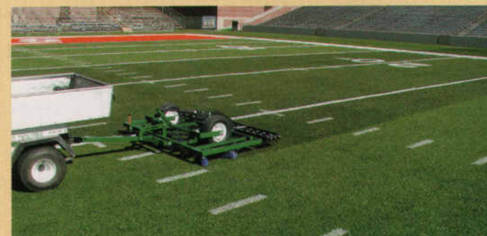
GreensSlicer Spring Tine Rake 3 rows of 28 tines.
