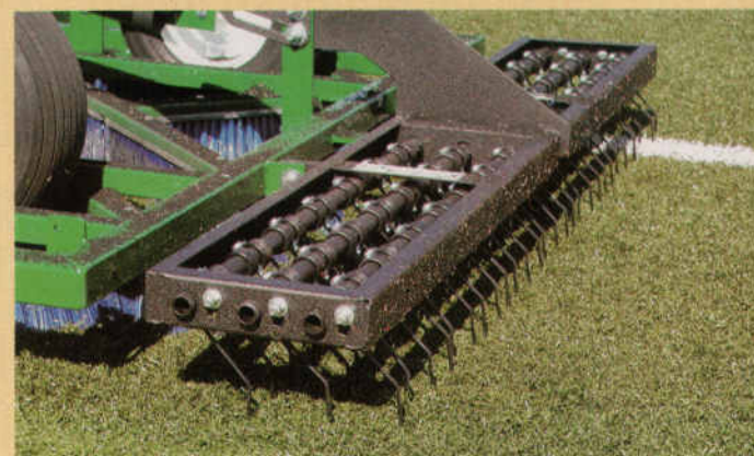
GreensSlicer Spring Tine Rake 3 rows of 28 tines.
