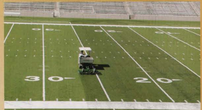
GreensSlicer Spring Tine Rake 3 rows of 28 tines.
