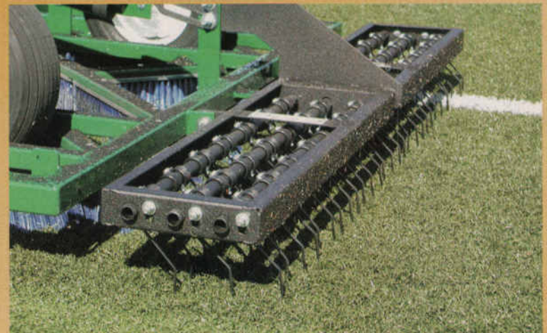
Greenslicer Spring Tine Rake 3 rows of 28 tines.
