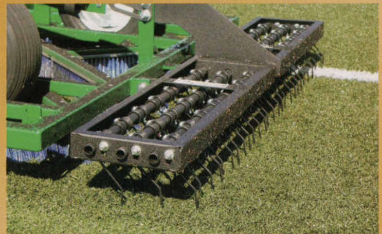
GreensSlicer Spring Tine Rake 3 rows of 28 tines.
