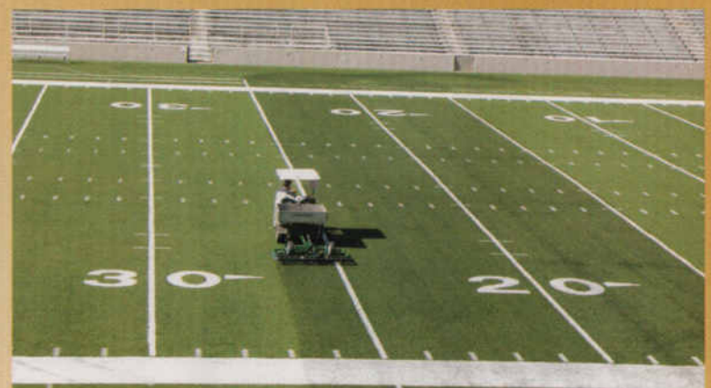
GreensSlicer Spring Tine Rake 3 rows of 28 tines.
