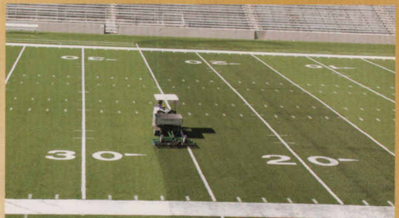
GreensSlicer Spring Tine Rake 3 rows of 28 tines.
