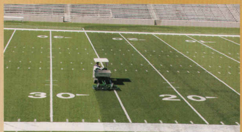
GreensSlicer Spring Tine Rake 3 rows of 28 tines.
