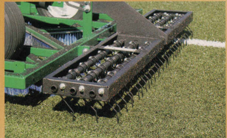
GreensSlicer Spring Tine Rake 3 rows of 28 tines.
