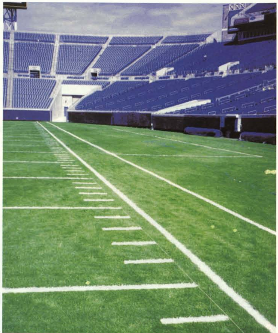
Precise field lines are created by running string from end zone to end zone.
