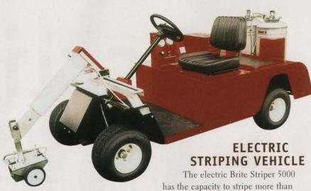
has the capacity to stripe more than 100 football fields with one charge, and manufacturer Pioneer says it provides the straightest lines of any field striper.
