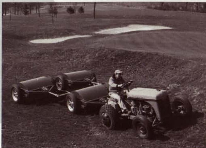
The first tractor-drawn tri-aerifier, developed by Tom Mascaro and used on athletic fields-circa 1950's.
