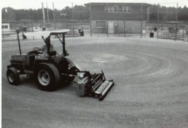
Outfield Aerator/Overseeder All with the same machine
