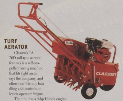
removable 50-lb. weight bar, a guard to keep cores, grass or leaves away from chain and sprockets, and fits through a 42-in. gate without removing the rear wheels.
