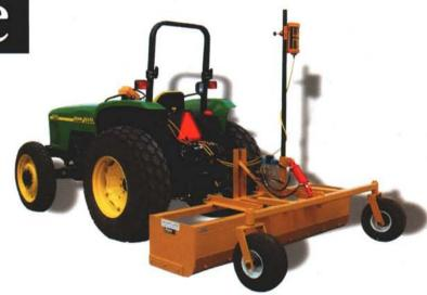
Laser Leveling is proud to introduce the first and only laser grading system designed specifically for baseball and softball field grading and finishing. Our Diamond Series family of cone-grade lasers allow you to dial in the exact amount of cone slope, meaning that your fields will always be perfectly graded, without ever moving the laser. The Diamond Series is quite simply the best solution available to ballfield construction and maintenance contractors on the market today.
