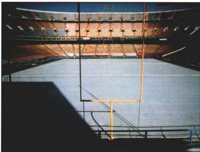
A turf blanket protects turf in winter at Denver's Mile High Stadium. Courtesy: Covermaster Inc.
