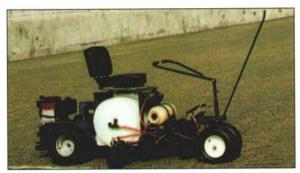
The Javdee Drive Liner is a self-propelled riding line marker. The 35-gallon paint tank carries enough marking material for a complete game field, or several practice fields. The 2-gallon flush tank cleans the discharge lines for work breaks, travel, or overnight. The center or side-mark spray shields are always operator-visible. A nearly zero turning radius reduces or eliminates back and turn maneuvers.
