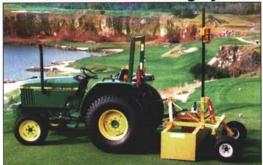
For level, single, or dual grade, GRADEMASTER is automatically laser controlled and eliminates uneven grade, potholes, wet spots and dips on athletic fields, greens or tee boxes. GRADEMASTER . . . The Right Choice for your Grading applications.
