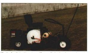
The Jaydee Drive Liner is a self-propelled riding line marker. The 35-gallon paint tank carries enough marking material for a complete game field, or several practice fields. The 2-gallon flush tank cleans the discharge lines for work breaks, travel, or overnight. The center or side-mark spray shields are always operator-visible. A nearly zero turning radius reduces or eliminates back and turn maneuvers.
