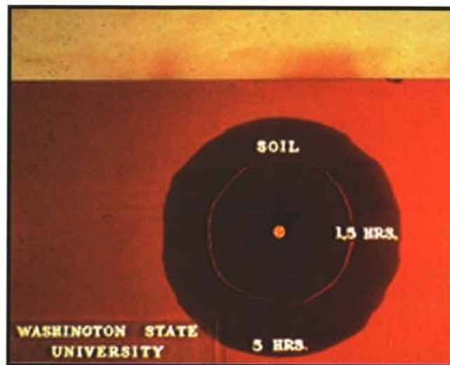
Capillary and adsorptive forces combine to pull water through a soil profile in movements independent of gravity. Courtesy: Lanco
