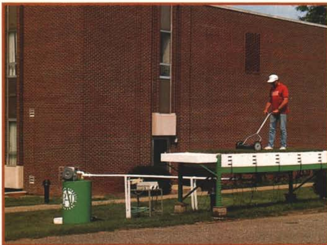
Ohio State University constructed a model of a section of PAT field to determine the effectiveness of vacuum-assisted drainage. Courtesy: Ken Chamberlain
