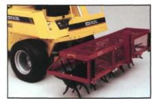
Unique up-front mounted core aerators help grounds managers get more production from their John Deere, Kubota, Ford, and Excel Hustler mowers. Millcreek core plug aerators have a protective safety cage, and individually mounted spoon wheels to allow easier turning without damage to turf. Affordable Millcreek aerators come in wide variety of sizes and styles in addition to the front-mounted units.
