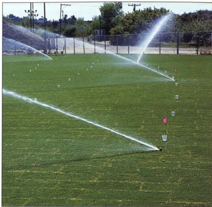
Precipitation rate is measured through catch cans placed near the sprinkler and halfway to the next one. The testing run time should be enough to collect 25 ml of water.
