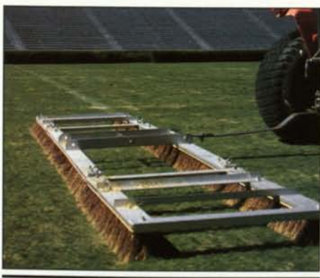
Auburn University's crew at Jordan-Hare Stadium brushes perennial ryegrass seed into their Tifway bermudagrass. Photo courtesy: Coleman Ward, Auburn University.
