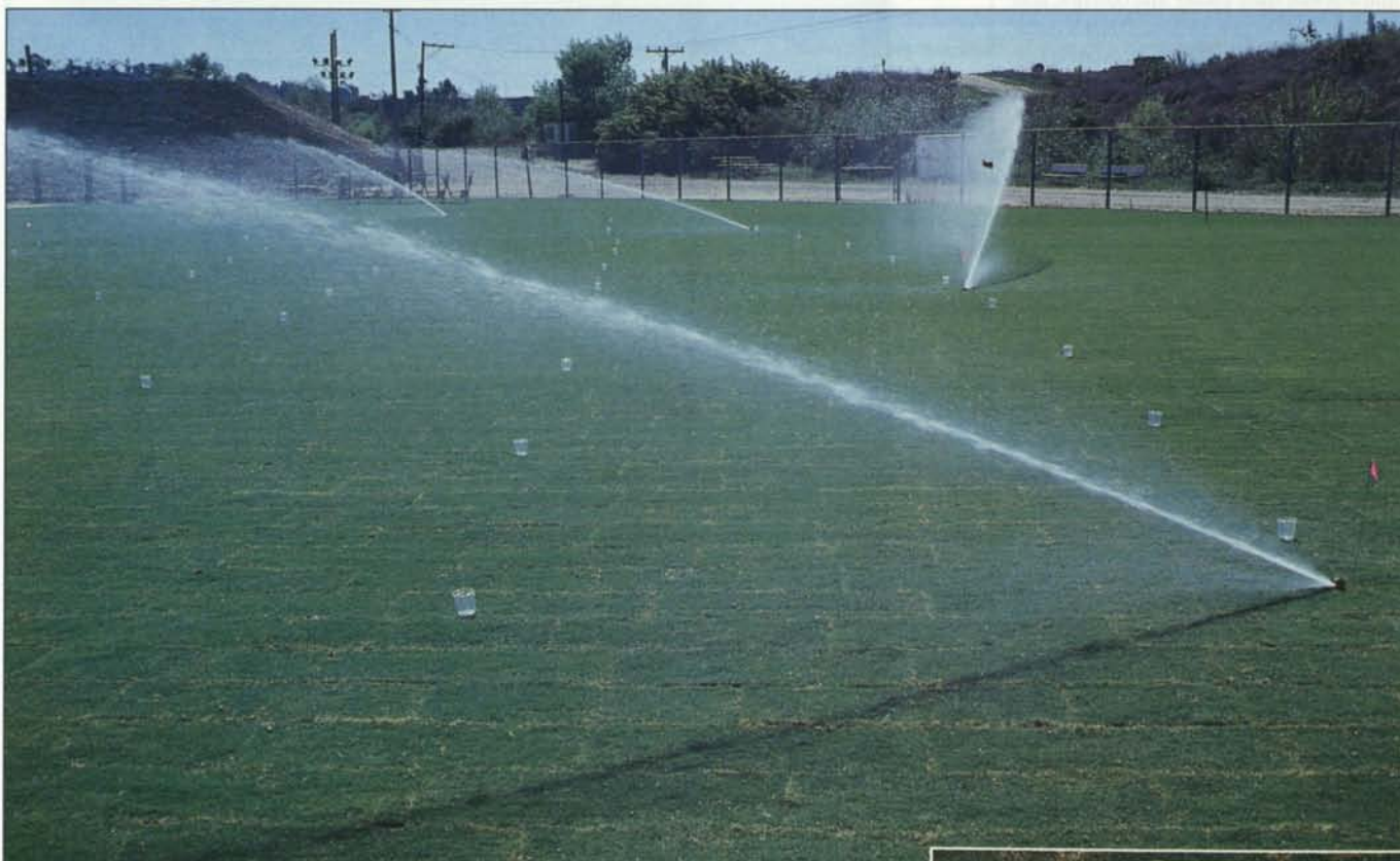
A typical grid layout for a catch-can test. Photo courtesy: David Shaw, University of California Cooperative Extension.
