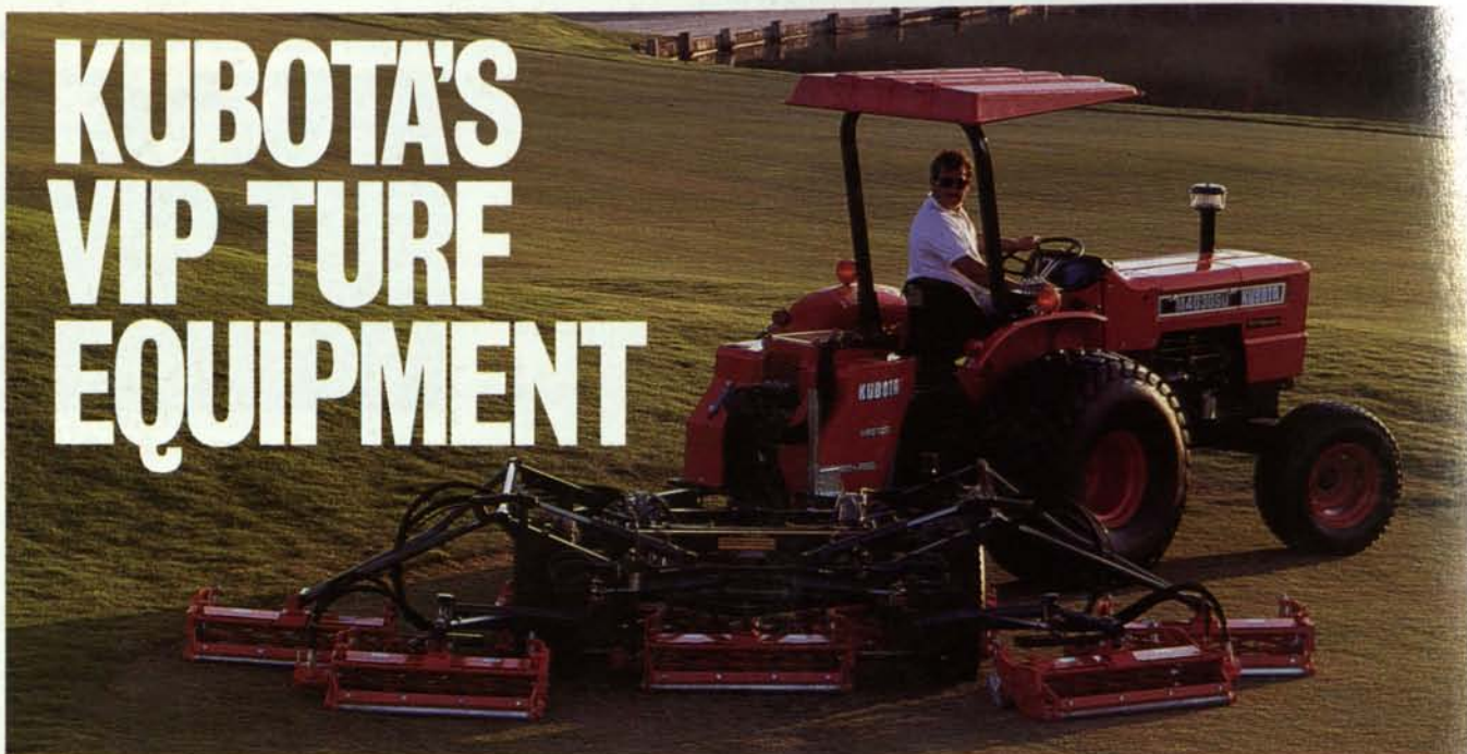
M4030SU with 5-gang Verti-Reel for high production mowing.
