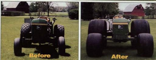
• Top Dressing • Spraying • Mowing • Back Filling Traps • Aerating The large contact area of the flotation tire effectively distributes load over a broad area. This produces lower unit ground pressure resulting in minimized soil compaction.
