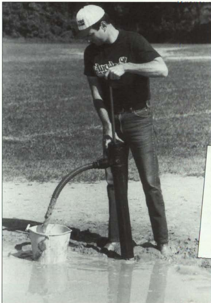
A hand pump solves many small drainage problems. Photo courtesy: Kuranda, U.S.A.
