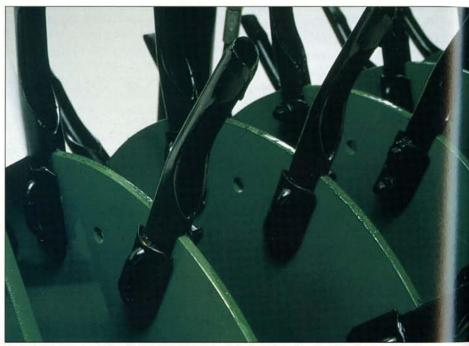
In addition to a host of aerators that can reach various depths, there are a number of tine options, from hollow to slicing, that can be used to address sitespecific problems. Photos courtesy: John Deere Company.
