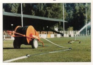
Rainboy reel irrigator is an economical, efficient solution to sports turf irrigation. The portable, above ground, easy tow design features the efficiency and accuracy of a retraction speed, regulated and controlled water turbine drive. Smooth and constant rotation of the retraction system provides quicker retraction speeds with uniform water application. For more information contact Jim Brown,
