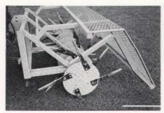
Sisis, Inc., Turf Equipment offers its Model DP/36 tractor mounted heavy duty aerator to relieve deep compaction and improve surface drainage on relatively flat areas with tractors capable of lifting 1,000 lbs. on the three-point hydraulic linkage.
