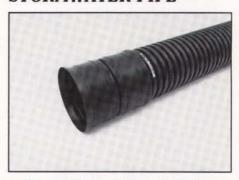
Hancor's high-capacity smooth interior storm drainage pipe is constructed of polyethylene. It features a corrugated exterior for strength, a smooth interior for high capacity, and a bell-and-spigot connection for watertightness. It can be used for stormwater drainage, cross drains and culverts, and retention/detention systems.
