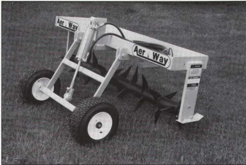
Holland Aerway fractures subsurface layers of soil.
