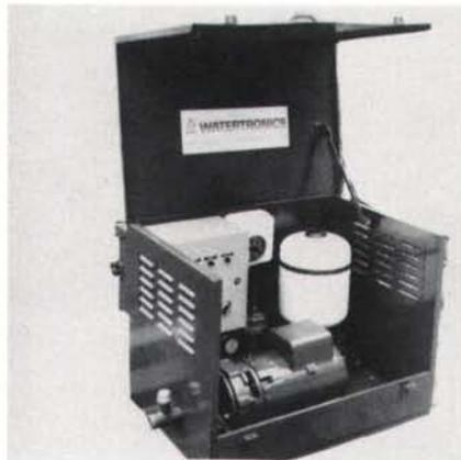
Designed for sports turf projects or boosting water pressure on golf courses, Watertronics' pumping station features a high-efficiency pump and motor, exterior fusible disconnect, interior pump controls, pressure gauge and switch, flow switch, and
