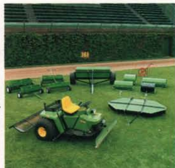
Attachments like spreaders, seeders, rollers, brushes, scarifiers, a wide blade and field finisher help the 1200 shine on the field.
