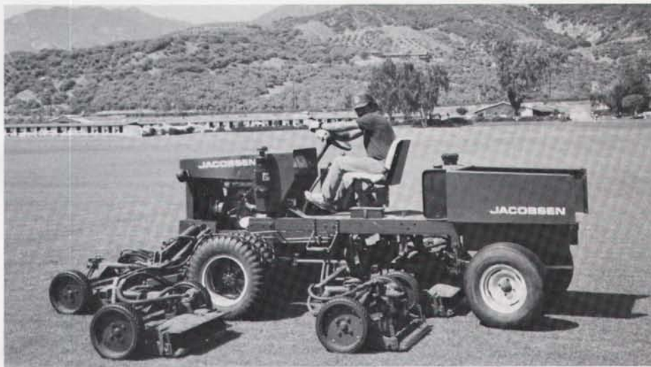
A Jacobsen HF-15 is used to mow the fields at Santa Barbara.
