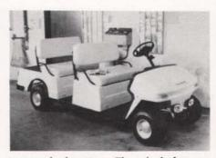
gage, and other items. The vehicle features a lightweight, two-cycle engine that requires no oil changes. It also has a lift-out battery pack tray for continuous use and an on-board automatic electric charger.
